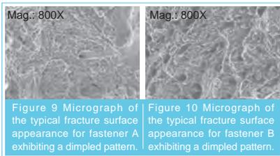
Figure 9 Micrograph of the typical fracture surface appearance for fastener A exhibiting a dimpled pattern.
