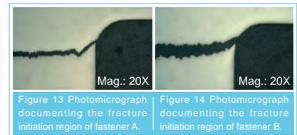
Figure 13 Photomicrograph documenting the fracture initiation region of fastener A.
