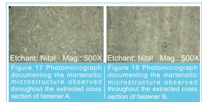
Figure 17 Photomicrograph documenting the martensitic microstructure observed throughout the extracted cross section of fastener A.
