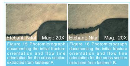
Figure 15 Photomicrograph documenting the initial fracture orientation and flow line orientation for the cross section extracted from fastener A.
