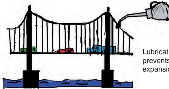
Lubrication of wire cables prevents fretting and oxide expansion corrosion
