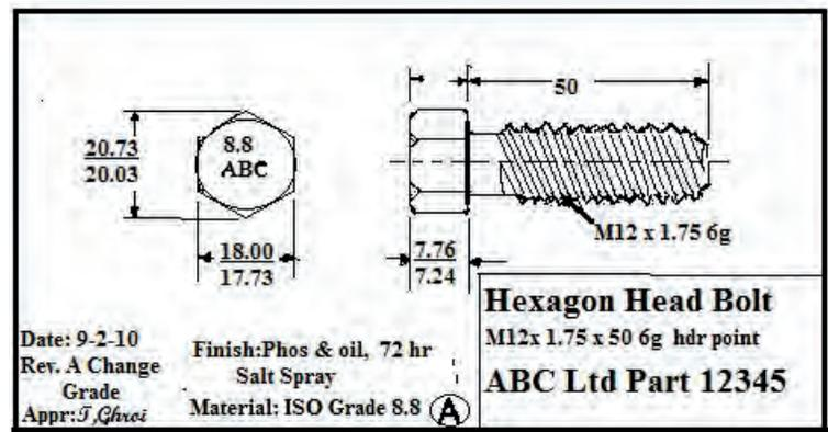
Fig. 2 Drawing for an Auto Part
