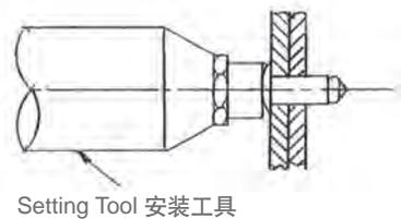
Fig. 3 A Tool Setting a Blind Rivet
