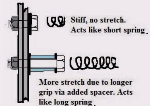
the joint strength on the high end, the bolt may go into bolt yield and permanent elongation may occur. This permanent additional lengthening of the bolt causes a reduction in cross sectional area. The reduced cross sectional area is less capable of carrying the load and cycle after cycle reduces the bolt strength until a failure caused by the hysteresis occurs.
