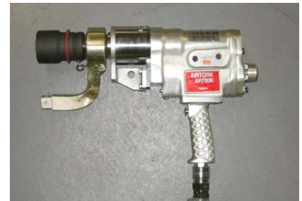
Fig. 3. Powered torque wrench
